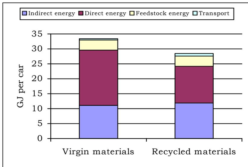
**Figure 2.** Gross energy requirement for Fiat Panda production using primary and secondary materials.
