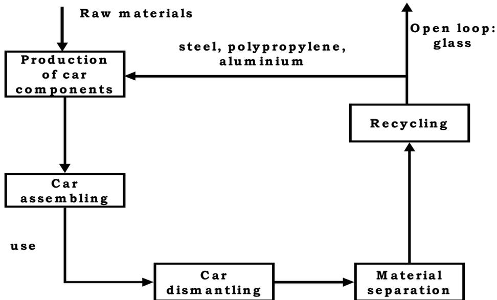
**Figure 1.** The materials flow in the Fiat Panda production system: the closed loop recycling includes steel, polypropylene and aluminium. Car glasses are addressed to an open loop recycling.
